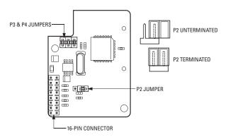
Figure 13. TXB-V Termination and Baud Rate (Bottom View)
